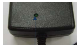
Power Indicator LED LED light turns: Red→Green→Yellow→No LED
