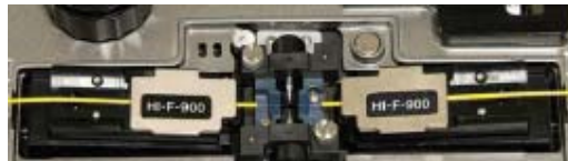
Splice with Fiber to Fiber
