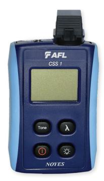
The NOYES CSS1-SM from AFL is a palm-sized, cost-effective dual LASER source designed for performing insertion loss measurements on single-mode fiber optic links when used with an optical power meter. When paired with an optical fiber identifier, the CSS1-SM may be used for fiber identification. The LASER output is stabilized to ensure accurate test results per current TIA/EIA requirements. Weighing only 0.4 lb, this light source is ideal for field use.
