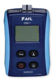
The NOYES CSS1-MM from AFL a palm-sized, cost-effective dual LED light source designed for performing insertion loss measurements on multimode fiber optic links when used with an optical power meter. When paired with an optical fiber identifier, the CSS1-MM may be used for fiber identification. The LED output is stabilized to ensure accurate test results per current TIA/EIA requirements. Weighing only 0.4 lb, this light source is ideal for field use.
