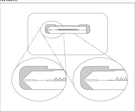
The technology of the Fibrlok II Optical Fiber Splice is also available in the revolutionary new Fibrlok Multi-Fiber Optical Fiber Splice (shown here in 12 fiber version).
