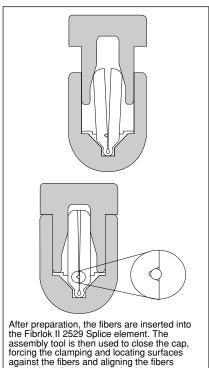
After preparation, the fibers are inserted into the Fibrlok II 2529 Splice element. The assembly tool is then used to close the cap, forcing the clamping and locating surfaces against the fibers and aligning the fibers precisely and permanently in place.
