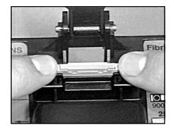
2.05 If using the 3M<sup>™</sup> Fibrlok<sup>™</sup> 2501 Assembly Tool, rotate the toggle arms for the appropriate fiber size.
